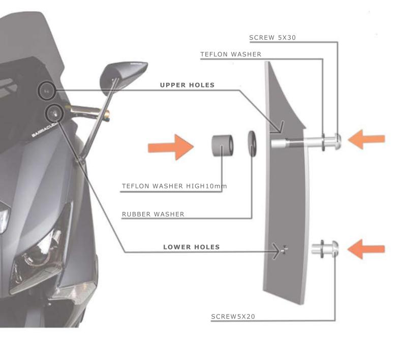
REMOVE THE ORIGINAL WINDSHIELD/SCREEN AND APPROACH THE BARRACUDA WINDHSHIELD/SCREEN. MOUNT IT LIKE THE ISNTRUCTION USING THE SCREWS AND THICKNESS IN-CLUDED. USE THE ORIGINAL SCREW FOR FIXING THE LOWER PART OF PLEXIGLASS.
