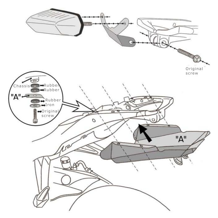
REMOVE THE ORIGINAL LICENCE PLATE FROM THE MOTORBIKE. APPLY THE BARRACUDA LICENCE PLATE LIKE SHOWN IN THE PICTURE.
