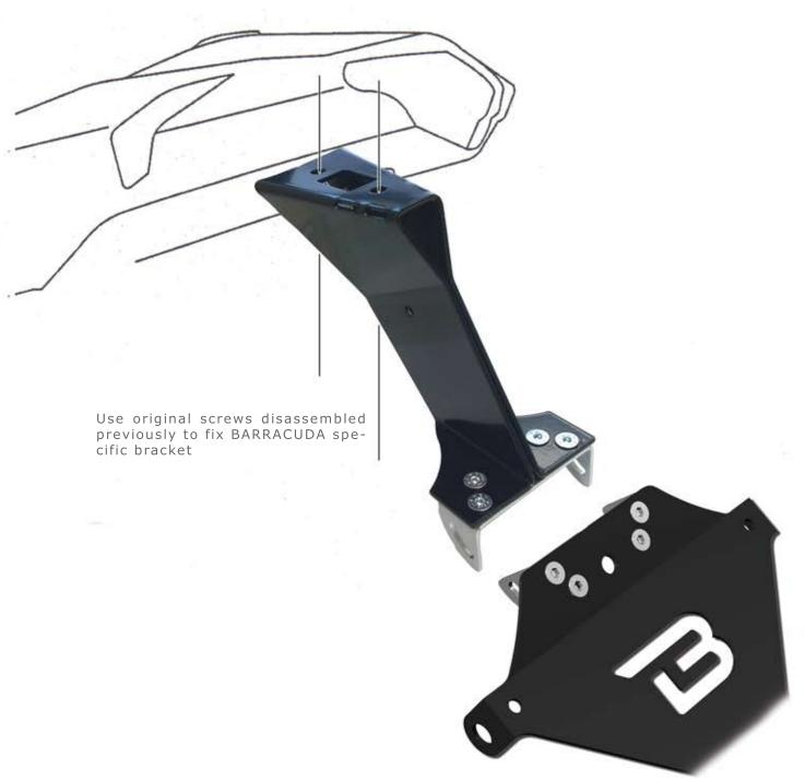
REMOVE THE EXHAUST AND THAN REMOVE THE PLATE THAT SUPPORT BOTH ORIGINAL LICENCE PLATE AND THE EXHAUST AND FIX WITH THE SCREWS JUST DISASSEMBLE TO THE BARRACUDA SPECIFIC BRACKET. REASSEMBLE EVERYTHING
